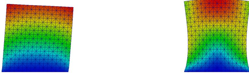
Figure 4.2: Deformed structures corresponding to the first (left) and second (right) lowest eigenfunctions for  $N = 16$ ,  $\nu = 0.49$ ,  $k = 3$  and  $\mathbf{a}_S = 1000$ . The color reflects the magnitude of the displacement field.
